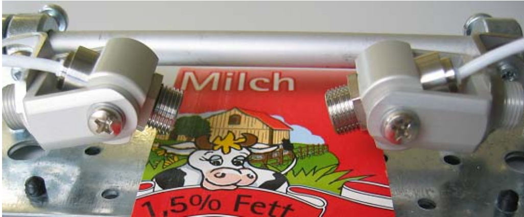
Fig. 6-1 possible adjustment of the sensor heads for the emission measurement
